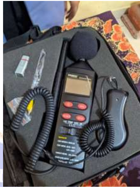
(Environtmental Meter (Light Meter, Temperature Meter, Humidity Meter, dan Sound Level Meter)
