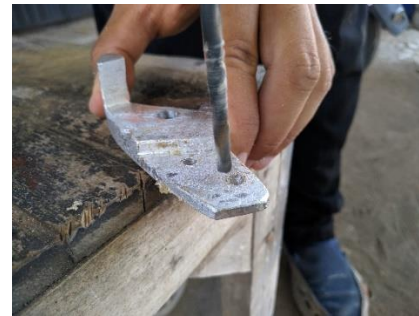
Gambar 63 Proses Pengeboran Anting Handle Rem
