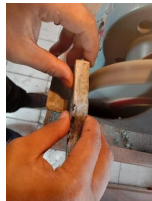
Gambar 29 Proses meratakan Handle Rem
