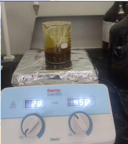
A laboratory hotplate (Thermo Scientific) is shown with a beaker containing a dark liquid. The hotplate's digital display shows a temperature of 29.0°C and a speed of 450 rpm. |
