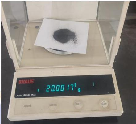
A digital analytical scale (OHAUS) is shown with a small white paper containing a dark, granular substance. The scale's display shows a mass of 20.0017g.                        |
