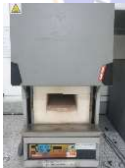
Furnace Pengabuan Batubara
