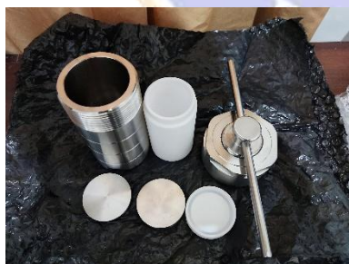
Alat hydrothermal autoclave
