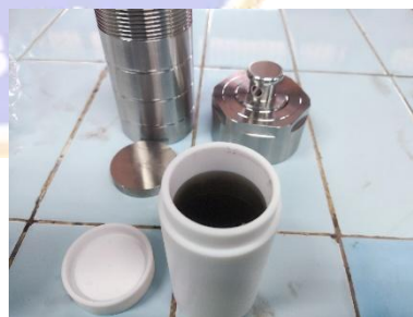
Sintesis CDs metode hydrothermal
