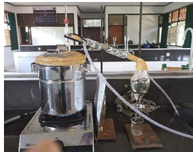
(b) Proses distilasi uap air
