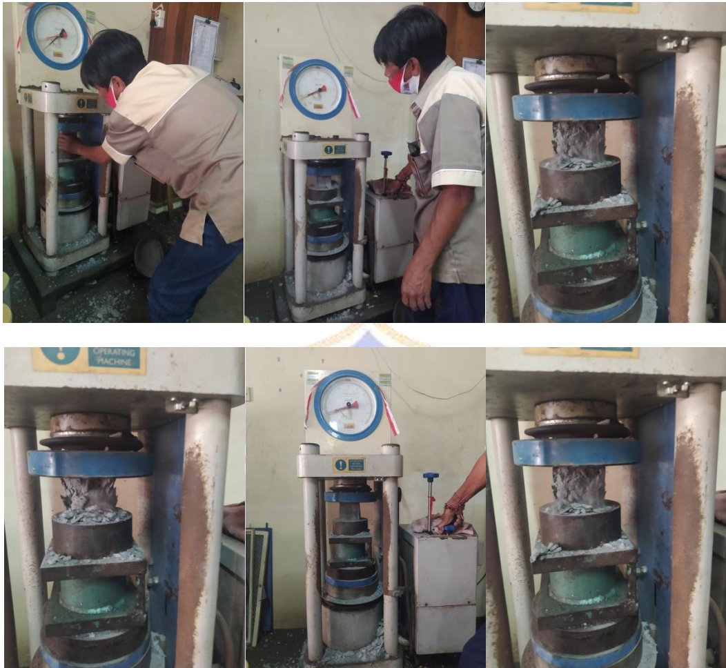
Lampiran 7. Pengujian Kuat Tekan Paving block
